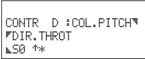
In the base types the switch S06 is assigned here as standard. If you assign ON instead of a switch, then throttle is **always** controlled via the transmitter control IDLE-UP - except during AUTO-ROTATION.
