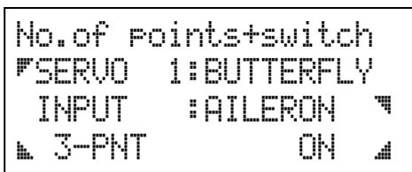
**Pressing the b** button opens the field for selecting a servo. Use the **q/n** buttons or the Digi-adjustor to leaf through the options.
