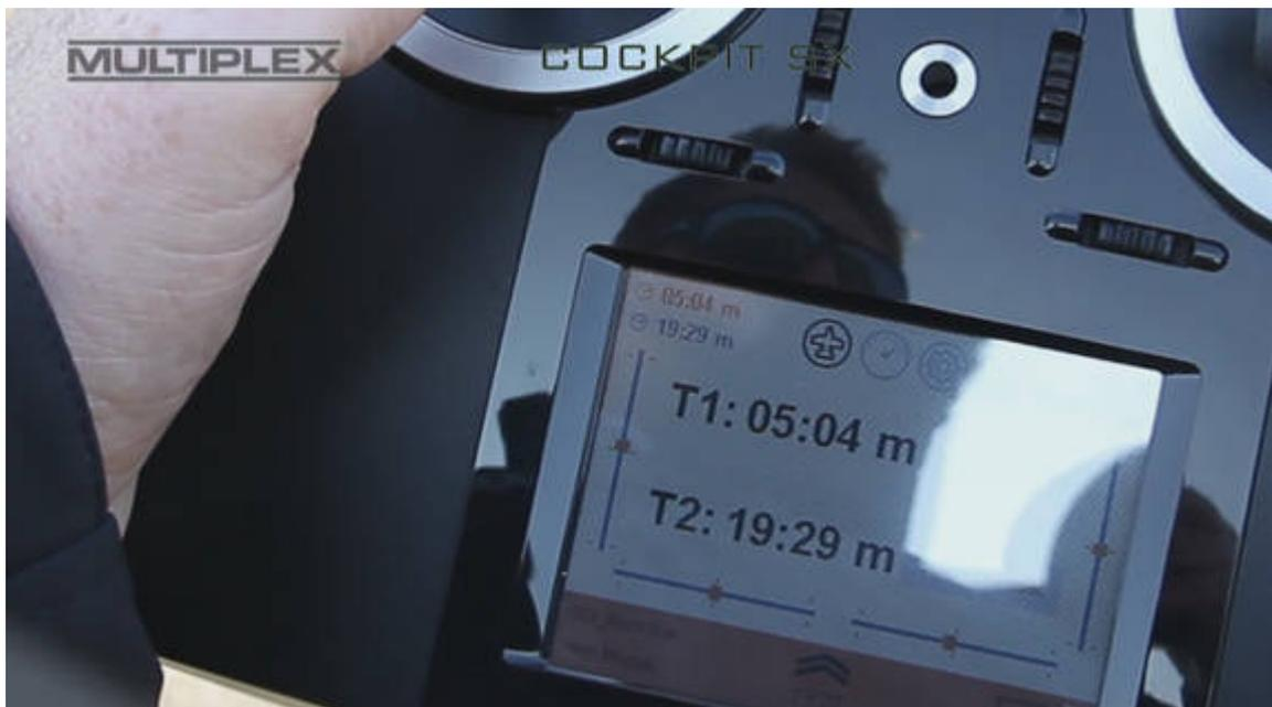
A place in the sun - with your COCKPIT SX. The integral screen is always clearly legible thanks to the automatic day / night switching. In fact, switching off the backlighting in sunlight saves so much battery capacity that the transmitter is capable of operating for up to 24 hours. This means that you can devote the whole day to what you really want to do - i.e. fly your models - without worrying, and, in particular, without the need for a battery charger.
