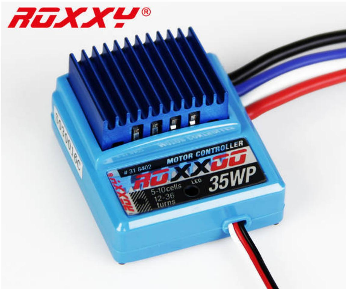
Speed controller for model cars and boats fitted with 540-size standard and "tuning" motors with 35 A = from 12 turns, 25 A = from 15 turns, 20 A = from 16 turns.
