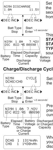
Set the discharge current on the left and the voltage cutoff on the right by pressing the **START/ENTER** key for more than 3 seconds to start the program. Discharge current can be set from 0.1-1.0A and voltage cutoff from 0.1-25.0V.
