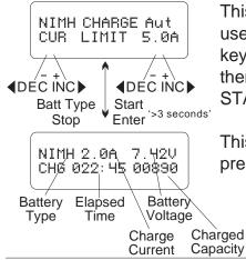
This program is for charging NiCd/NiMH batteries typically used in an R/C model application. Press the START/ENTER key until the parameter you want to change begins to blink then use the INC or DEC keys to change the value. Press the START/ENTER key to store the setting.
