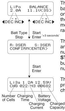
The first line on the left side of this screen shows the type of battery chosen. The second line shows the user set current on the left and the user set voltage on the rights. After setting the current and voltage, press the **START/ENTER** key for more than 3 seconds to start the process (charge current range: 0.1-6.0A, voltage range: 3.7-22.2V).
