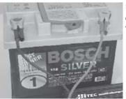
Using terminal clip attaching to car battery.
