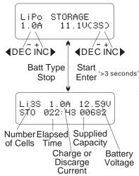
This screen, you can set up the current and voltage of the battery pack. Charging and discharging will bring the batteries to the storage level.
