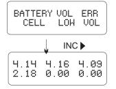
This screen shows that the processor detected the voltage of one on the cells is too low.
