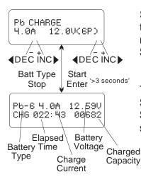
Set the charge current on the left and the nominal voltage on the right. Charge current can be set from 0.1-6.0A. The voltage must match the battery being charged. Press the **START/ENTER** key for more than 3 seconds to start charging.
