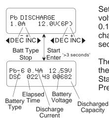
Set up the discharge current on the left and the nominal voltage on the right. The discharge current can be set from 0.1-1.0A. The voltage should match the battery being charged. Press the **START/ENTER** key for more than 3 seconds to start discharging.
