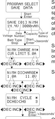
Setting of the parameters in the first screen will not affect the charge and discharge process. It is only for identifying the specification of the battery you will create a preset for. In this example it is a NiMH battery pack with 12 cells and a capacity of 3000mAh. When you have completed this process press and hold the **START/ENTER** key for 3 seconds to enter the charge/discharge setup screen.
