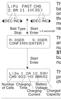
The first line on the left side of this screen shows the type of battery chosen. The second line shows the user set current on the left and the user set voltage on the rights. After setting the current and voltage, press the **START/ENTER** key for more than 3 seconds to start the process (charge current range: 0.1-6.0A, voltage range: 3.7-22.2V).
