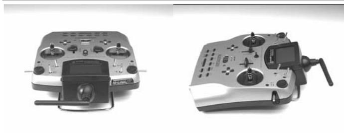
For applications where the model is not operated directly above or below the transmitter, the optimum aerial orientation is vertically upwards; this applies in particular to model cars and boats.
