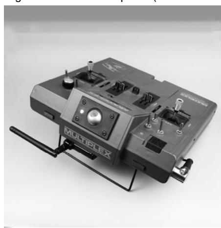
For applications where the model is not operated directly above or below the transmitter, the optimum aerial orientation is vertically upwards; this applies in particular to model cars and boats.
