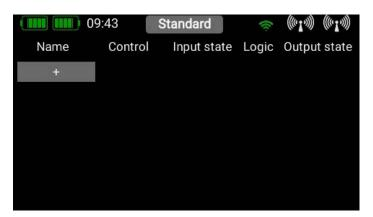
Select the **Virtual Switch** button in the menu, then press + to set up a new virtual switch. You can rename the virtual **switch** by pressing the switch button. As you can see, this field includes a small triangle at top right. This means that a function can be selected here by holding your finger on it. In this case the virtual switch can be erased again by holding your finger on the switch button.
