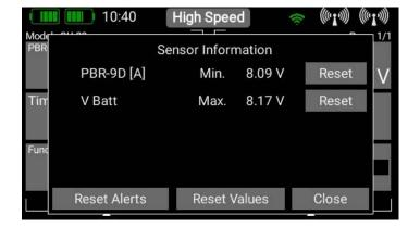
The recorded minimum and maximum values and alarms can be erased individually in each widget. If you wish to be able to erase all the alarms and all the minimum and maximum values at once, you can press the **Right-hand** button in the **Pull-down menu**. This action resets **all** values and alarms.
