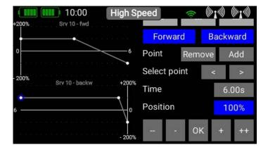
In this example the door would stay still for one second, then run from -100% to +100% over a period of one second. After a two-second pause, the door would run from +100% to -100%, again with a one-second delay. After a further second the sequence is complete.
