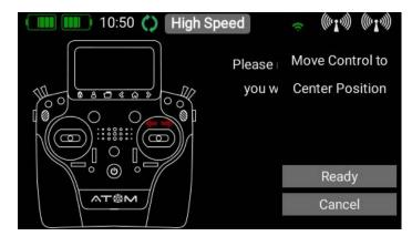
If you have installed a proportional control or a 3-position switch, you also need to move the transmitter control to the center. Touch Finished to complete the process. The **Direct** button can be used to reverse the transmitter control's direction of operation.
