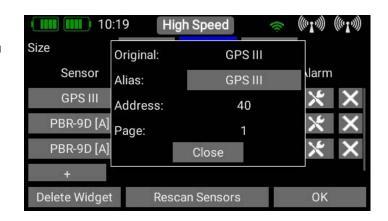
In this menu you can change the sensor name, and see the current sensor **Address**. To rename the sensor, open the keypad by pressing the field after **Alias**. Note that long sensor names, in particular, can result in extended spoken messages. If you are using M-Link sensors, the standard M-Link-XY can be changed to a more informative name. If you wish to restore the original name supplied by the sensor, simply erase all the characters in the Alias field, and confirm the empty field.
