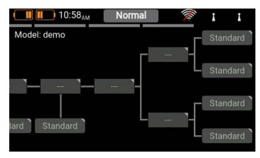
The most important thing to know at this point is that the **ATOM** prioritizes the flight modes. Priority runs from left to right, i.e. the flight modes in the left-hand tree diagram have the highest priority, and those on the right the lowest priority. Even when the flight mode structure is complex, this means that you can, for example, overrule all other switch positions with a single switch, returning you very quickly to "normal" flight mode.
