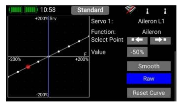
This is the procedure: use the arrow buttons to select the point you wish to adjust. Briefly press the displayed setting at **Value**, then adjust the servo for this position. The **Smooth button** can be used to even out the course of the curve. Right at the bottom you will find a **Reset button** which sets the curve back to a straight line. Once you have set the desired curve, return to the Servo Curve menu, where you will find three Preview buttons:
