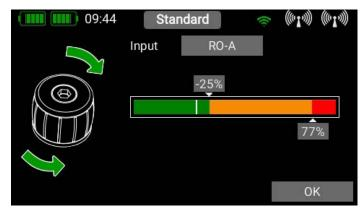
The two switching points can now be placed in any position you like by moving them with your finger. The red area indicates the "Off" state; the green area the "On" state. The orange area indicates "hysteresis", i.e. the area in which no switching takes place.
