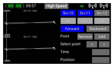
Below the **Srv.** buttons you will see two further buttons: **Forward** and **Reverse**. These buttons are also designed to display only those sequencer graphs which you wish to see or adjust at the moment.
