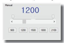
Once you have your desired Fail Safe position, click on the "FS-Position" button Fail Safe Test as seen in the illustration.
