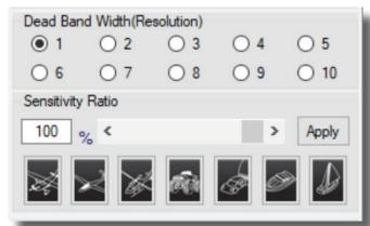
In addition to the manual adjustment method there are seven preset sensitivity settings for 3D Aircraft, Sailplanes, Helicopters, Off and On Road vehicles, Power Boats and Sail Boats
