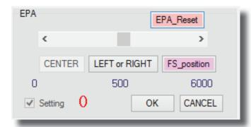
The first setting is the center point. When you have reached your desired center point click on "CENTER" to set this point and continue on to the left and right endpoints. Click "OK" when prompted by the pop-up screen.
