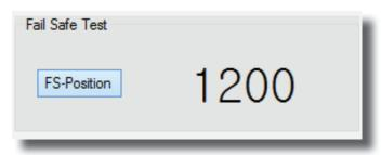
Generally, the servo will hold its last commanded position or enter into the programmed failsafe setting when the signal to the servo is lost. When FAIL SAFE Limp mode is enabled the servo will not hold a certain position when the signal is lost - in the instance the F/S or Hold function of the servo will not be activated.
