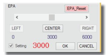
The first setting is the center point. When you have reached your desired center point, click on "CENTER" to set this point and continue on to the left and right endpoints. Click "OK" when prompted by the pop-up screen.
