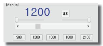
Once you have your desired Fail Safe position, click on the "FS-Position" button in the Fail Safe Test section to set the fail safe position. Once it is set, click the button again to exit the Fail Safe setup.
