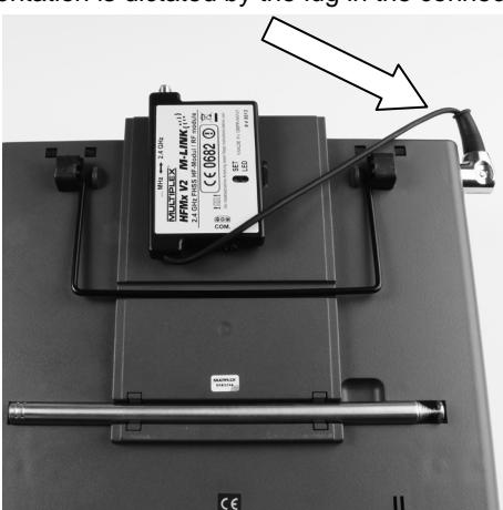
2. If the cable exits the connector in an awkward position, the internal part of the DIN plug (contacts and contact holder) can be rotated as follows:
