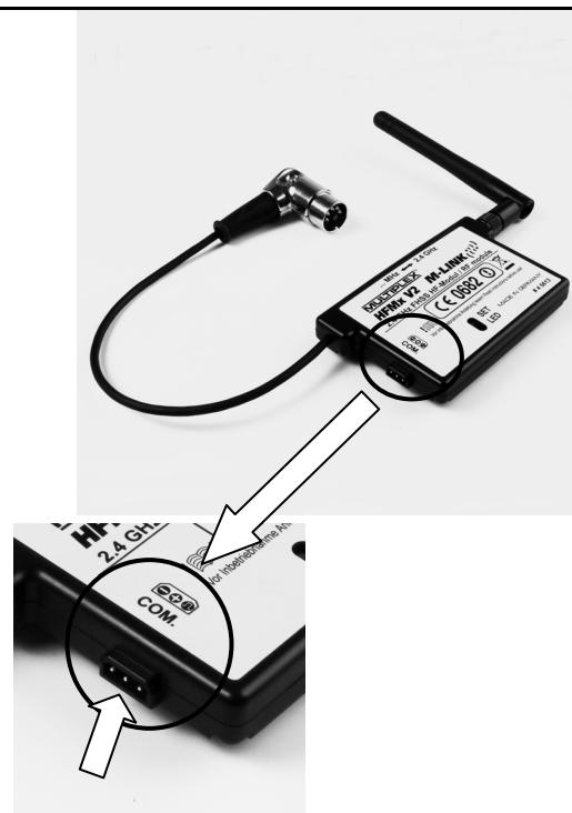
To update the firmware of the **HFMx V2 M-LINK 2.4 GHz RF module** you require the following items:
