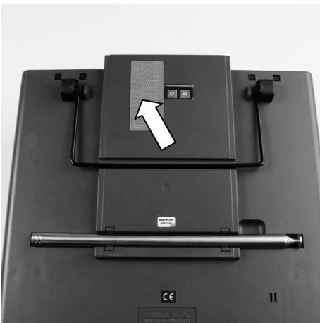
3. Attach the **HFMx V2 M-LINK 2.4 GHz RF module** to the transmitter case:
