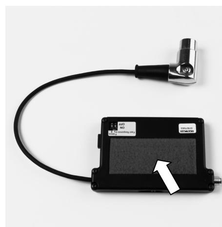
2. Stick the Velcro tape (hook side) to the transmitter case in the appropriate position:
