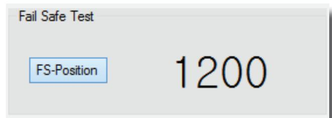
Generally, the servo will hold its last commanded position or enter into the programmed failsafe setting when the signal to the servo is lost. When FAIL SAFE Limp mode is enabled the servo will not hold a certain position when the signal is lost - in the instance the F/S or Hold function of the servo will not be activated.
