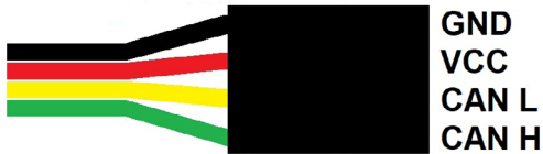
Pin layout of Hitec CAN actuators (not applicable to the SG-series)
