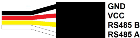
Pin layout of Hitec RS485 actuators*
