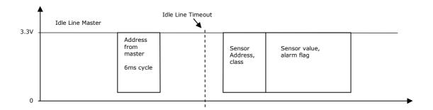
The sensor is slave. It receives bytes continuously until an idle line timeout occurs. After the timeout, the sensor interprets number and content of the received bytes. If the number of bytes is 1 (one) and this is a valid address or a broadcast command, the sensor responds with data or reacts to the command (see chapter 4.8 Addresses / commands).
